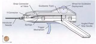
Figure 3. A diagram of the final device prototype.
