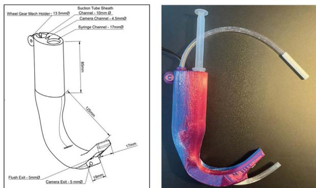
Figure 1. A mechanical drawing of the prototype laryngoscope and the functional prototype.
